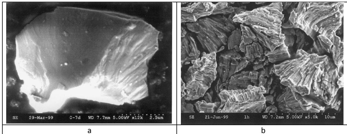
Figure 3. Scanning electron micrograph (SE-mode) of a) particles obtained by crushing nuclear fuel and b) particles obtained after annealing of  $\text{UO}_2$  in air at a temperature of  $400^\circ\text{C}$  for 1 h (b).
